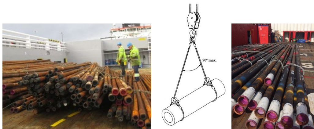
Figure 2: Business-as-usual wire sling system 1 . Sometimes also referred to as "bundling" 2
