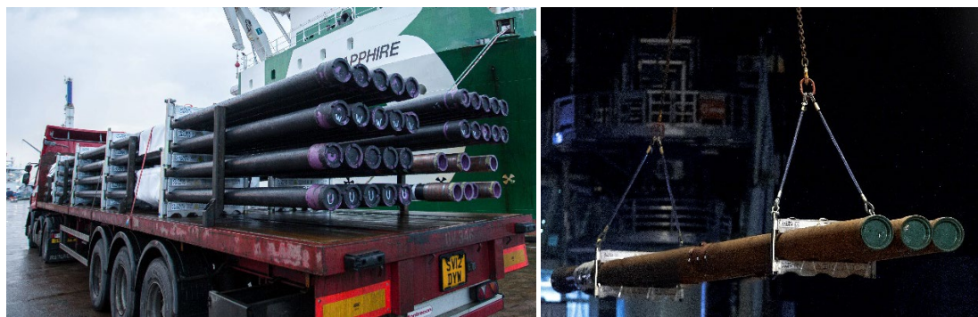
Figure 1: Pictures of Global Gravity's Tubular Transport Running System (TTRS) loaded with pipes on a truck and being transported with crane using wire slings unto an oil rig.
